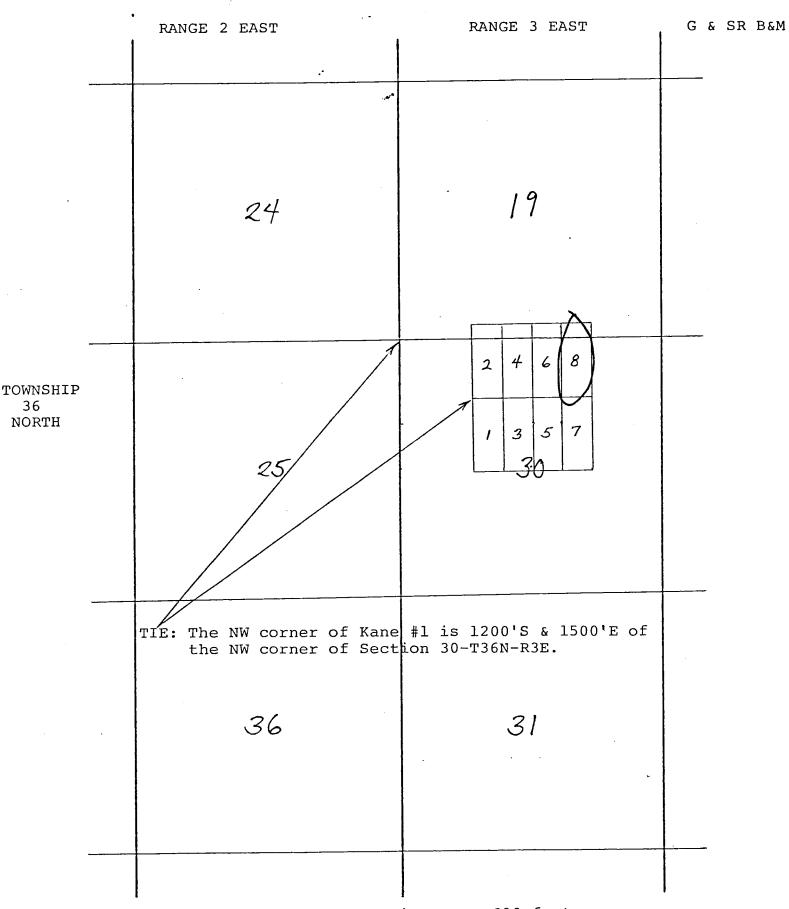
Side lines are 1500 feet, end lines are 600 feet; bearings are North/South, East/West parallel to the section lines except where noted.
